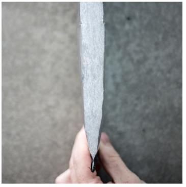
Inside is our hollow-fiber insulation – the SureTemp® brand's highest level of insulating material – between woven polyethylene layers.
